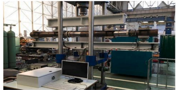
Fig. 4. Pipe Fatigue Test Under Cyclic Load
